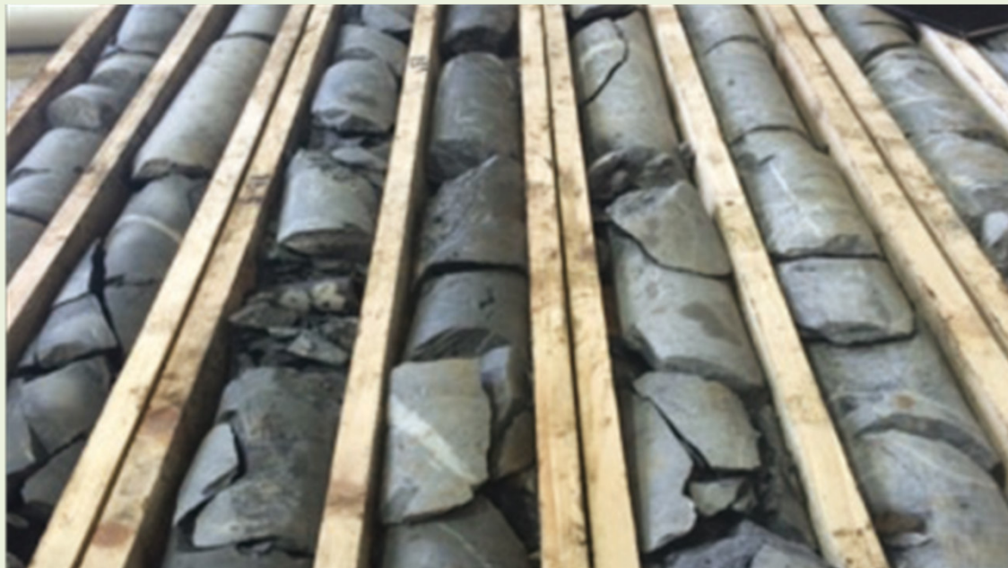
Clontibret Core : 2.5m @ 25 g/t Au in a pervasive sericite/white mica and carbonate alteration zone
