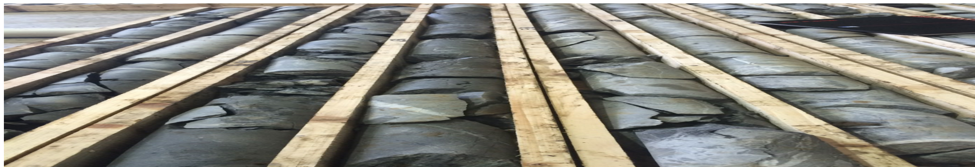
Clontibret gold mineralised drill core (2.5m @ 25 g/t Au)
